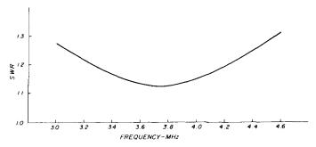
fig. 12. Calculated SWR at the input of the Wilkinson hybrid using 75-ohm cables. Each leg was terminated in a 50-ohm resistive load.
